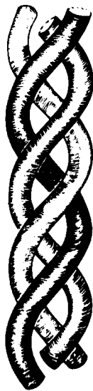
Figure 3. Cooperative twist deformation of a bundle of three chains (see text). In the instance shown the regularity of the deformation gives rise to a triple helix.
